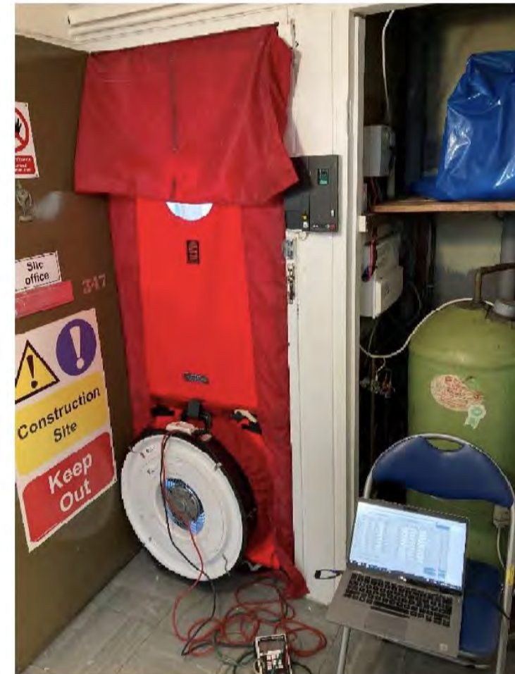
Figure 2: Test set-up showing the blower door mounted in the front door.
