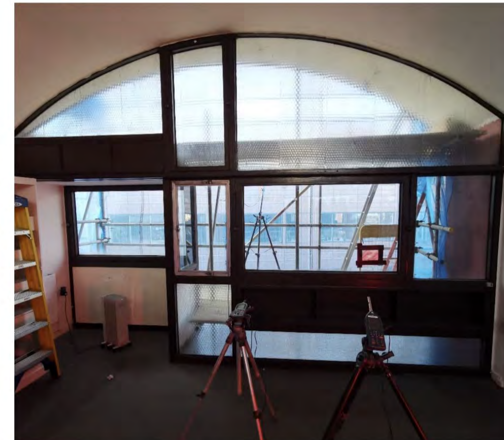
Photograph 1: Two sound level meters set up internally with window system under test.
