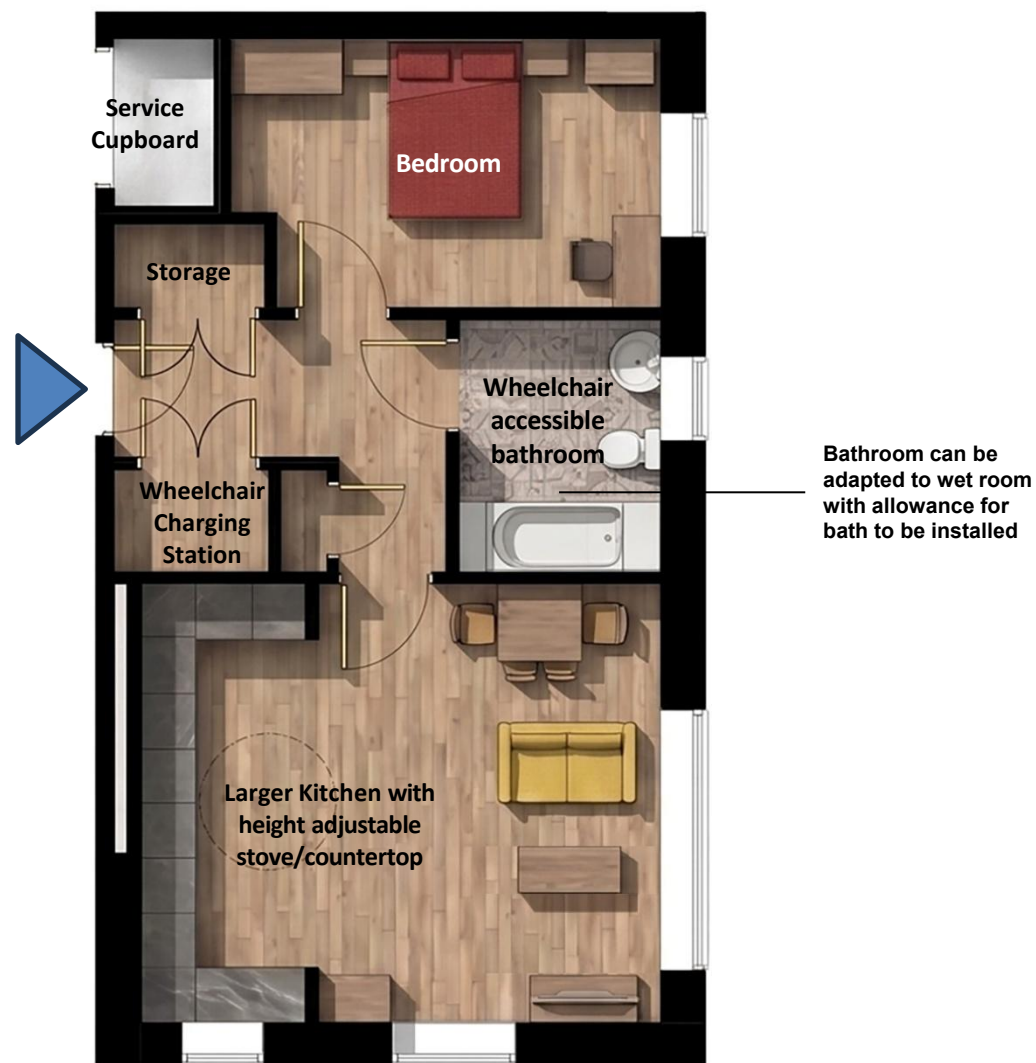
Proposed M4(3) Unit 1 Bedroom Apartment Wheelchair Accessible
